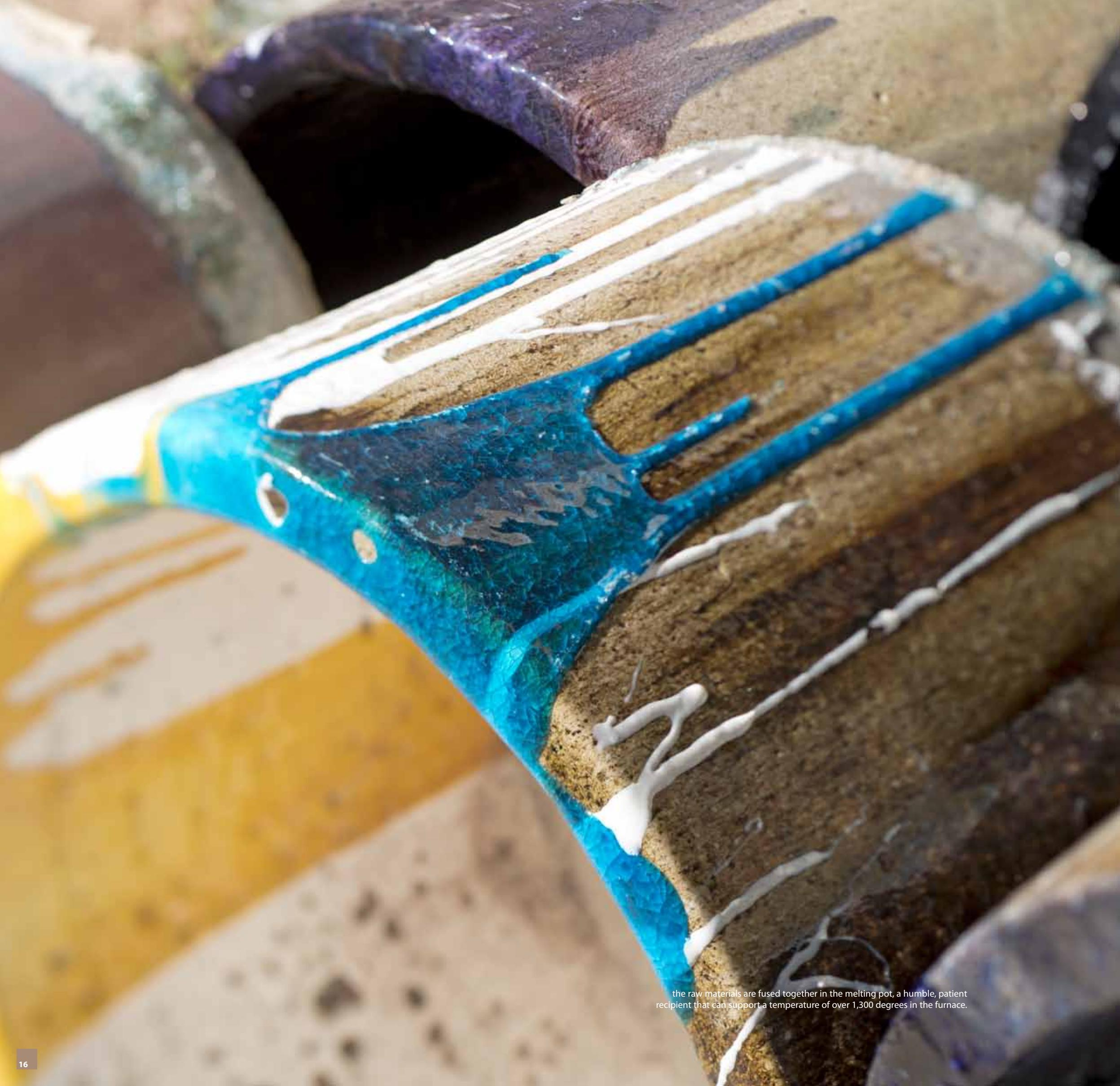
the raw materials are fused together in the melting pot, a humble, patient recipient that can support a temperature of over 1,300 degrees in the furnace.
